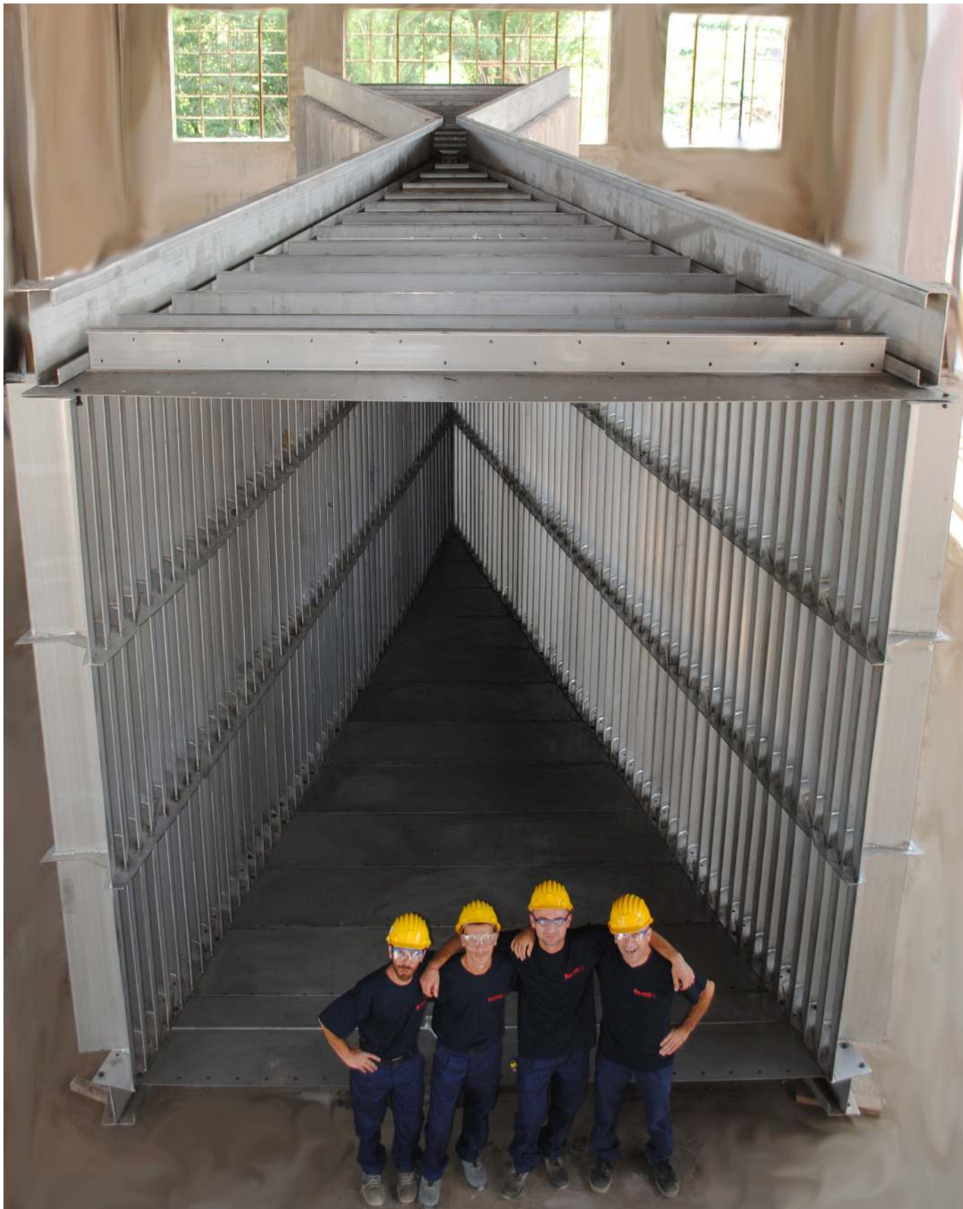
Vacuum Tower - Feed Inlet Vane Distributor Column diameter 16.000 mm - Nozzles diameter 3.600 mm
